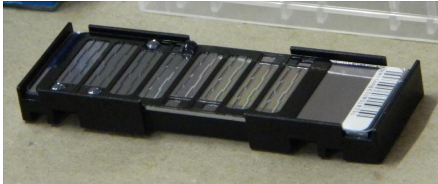
Figura 1. Bovine HD Genotyping BeadChip 777k (Illumina Inc., San Diego, CA)
