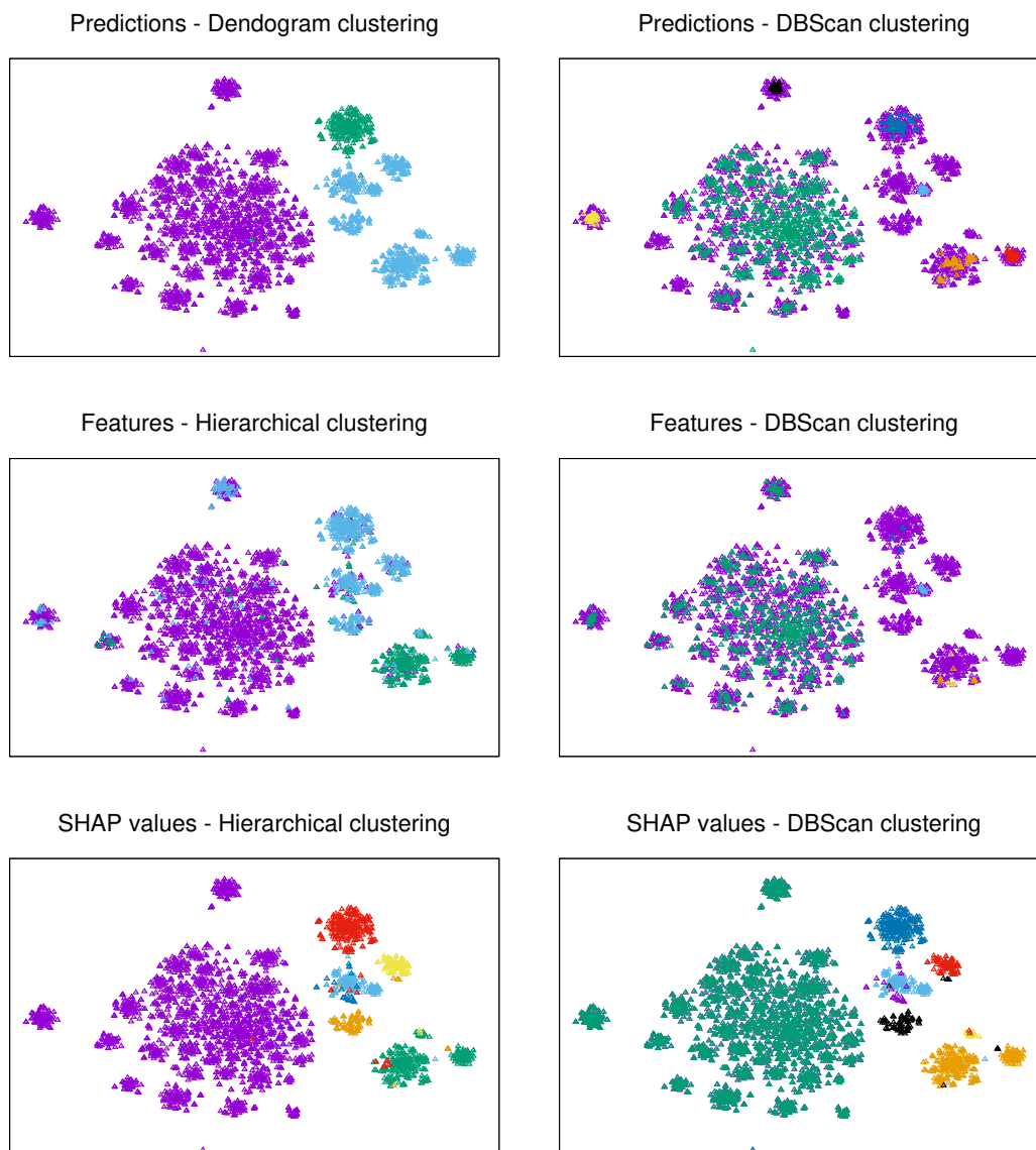
Figure 4.6: (Color online) T-SNE visualization of the model space after being clustered using different clustering algorithms and different criteria. Different colors mark different clusters. All clustering parameters were selected by maximizing the silhouette value in the model preference space. Models were built using Extreme Gradient Boosting (aka XGBoost). Silhouette values: Predictions = (0.17, 0.01); Features = (0.05, 0.03); SHAP values = (0.83, 0.95), respectively for Dendrogram clustering and DBScan clustering.
