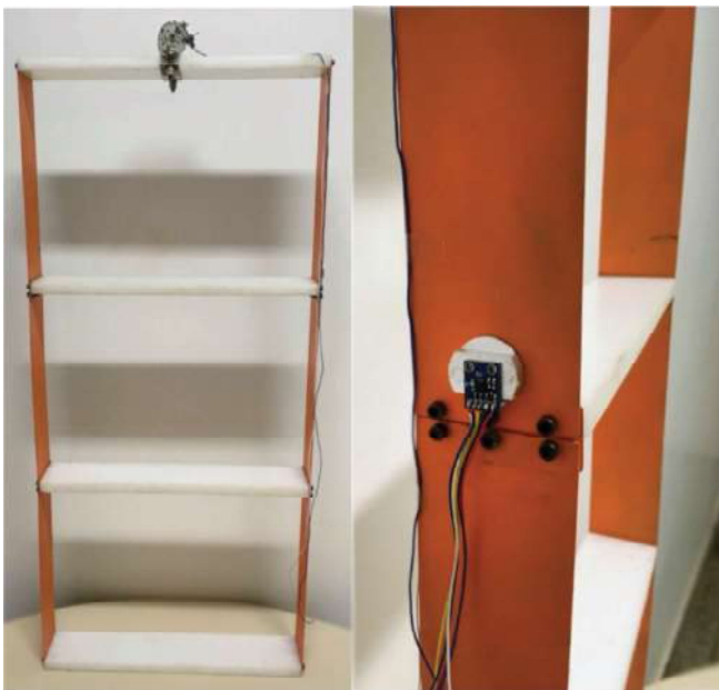
Figure 3: Mechanical system studied (Three story shear building).
