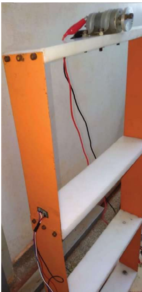
Figure 5: Location of the accelerometer sensor.
